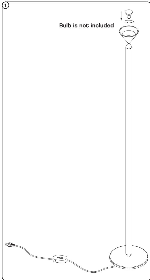
Plug in the power supply of AC 230V 50/60Hz;
