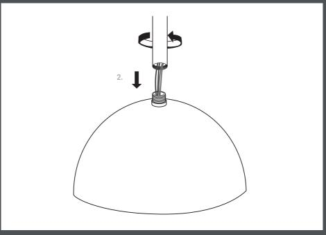
Install the lamp post on the base and tighten it in the direction shown in the drawing
