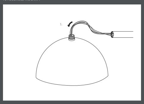
1. Route the wires down into the base so they are out of the way.
