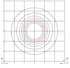
Efficiency 54.87 lm/W Coordinate System CG **Total Flux** 811.58 lm Maximum Value 173.75 cd
