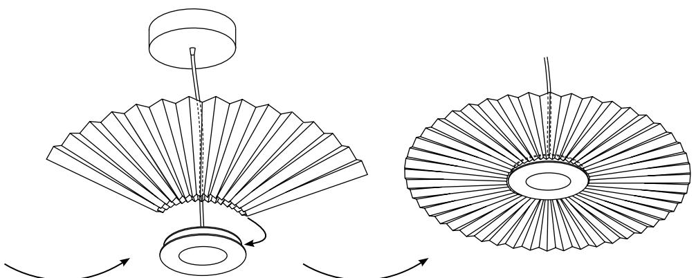
Thread the canopy and the cord through the pleated shade. The seam should be on the inside. Place the assembly on a flat surface, insert the pleated shade into the slot of the light fixture block, and press outward to flatten the shade. Two people are needed to properly flatten the shade.
