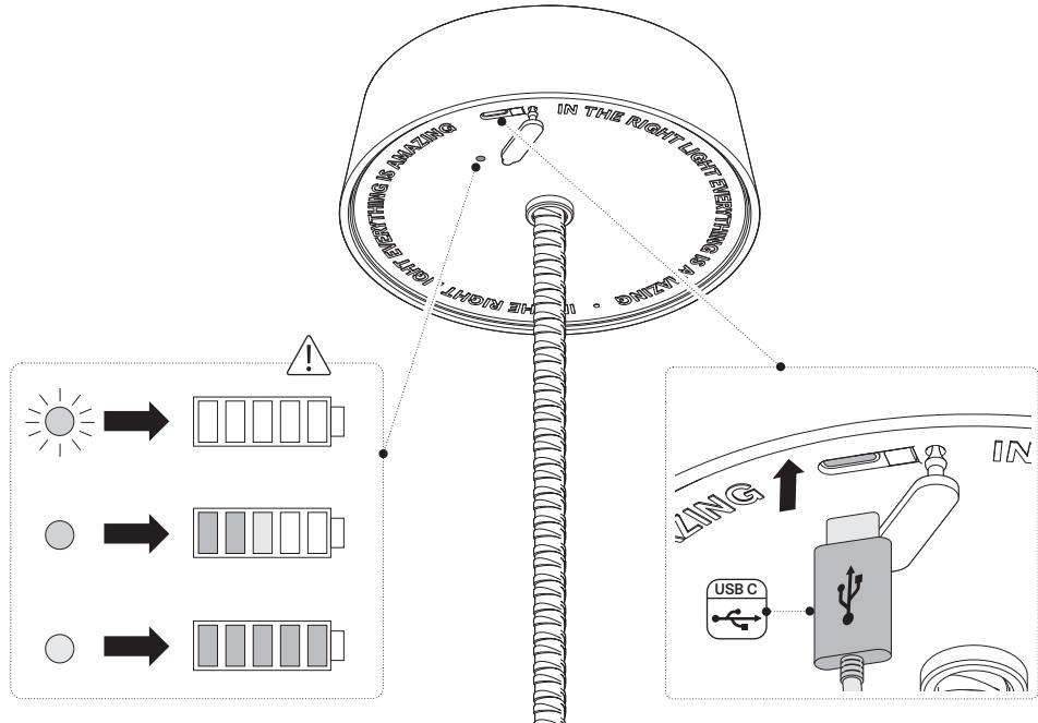
**EN** Red LED: will flash when the total hours of use have been reached. Recharge with the cable provided.
