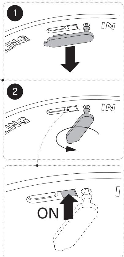
**EN** When using for the first time, activate the switch to connect the battery. In the event of a dimmer malfunction, press the button to reset the touch sensor.
