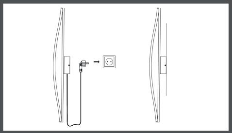
Plug the socket into a power outlet. If there is a built in lamp socket in the wall, the lamp can also be mounted directly to the wall without the cable.
