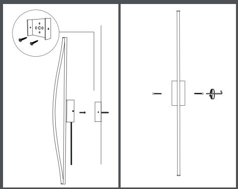
1. Detach the mounting plate from the wall lamp and mount it to the wall. Make sure to use appropriate screws and rawlplugs/anchors. Mount the wall lamp to the plate on the wall using the plated screws. Turn the screws clockwise for fastening.
