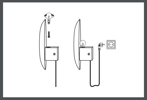
2. Place a recommended light bulb in the E14 socket. Plug the socket into a power outlet. If there is a built in lamp socket in the wall, the lamp can also be mounted directly to the wall without the cable.
