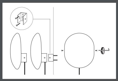
Detach the mounting plate from the wall lamp and mount it to the wall. Make sure to use appropriate screws
