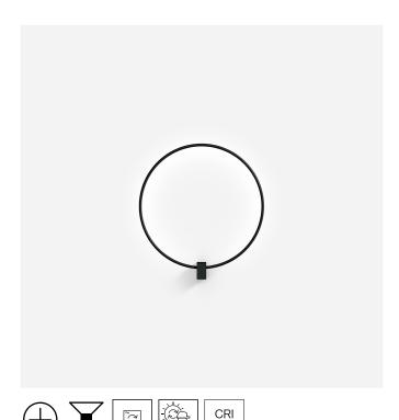
Round wall surface luminaire made from aluminium; indirect light distribution; surface Black Matt; powder coated, matt texture; RAL 9005; opal PMMA diffuser; PCB 3-step binning; phase-cut dim; light colour 3000 K; binning initial MacAdam ≤ 3 SDCM; CRI ≥ 90; 220 - 240 V; degree of protection IP20; Class 1; driver included; optional spacer available for overlapping; light source replaceable by Wever & Ducré or by a professional with explicit authorization; control gear replaceable by end-user;
