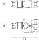
Junction - IP68 rated 3-way terminal box for electric cable connection
