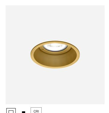
Round ceiling recessed downlight made from die-cast aluminium; surface Gold; wet painted, matt smooth; installation without tools using wire springs; suitable for ceiling thickness of 4-27 mm; recessed depth 115 mm; lamp socket GU10; lamp type PAR16; max. 12W; 100 - 240 V; degree of protection IP20; Class 2; lamp not included;
