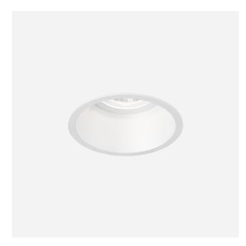
Round ceiling recessed downlight made from die-cast aluminium; surface White Matt; powder coated, matt texture; RAL 9010; installation without tools using wire springs; recessed depth 90 mm; with COB (Chip on Board) technology for maximum efficiency; light colour 3000 K; binning initial MacAdam  $\leq$  2 SDCM; CRI  $\geq$  90; beam angle 34°; degree of protection IP20; Class 3; driver not included; light source replaceable by Wever & Ducré or by a professional with explicit authorization;
