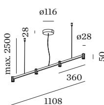
[253564CH5] The technical data represent rated values for an ambient temperature of 25°C. The data values for the luminous flux are initially subject to a tolerance of +/- 10%, those for the electrical connected load are initially subject to a tolerance of +/- 10%, and those for the colour temperature are initially subject to a tolerance of +/- 150 K. No liability is assumed for typographical or printing errors. The general terms and conditions of Wever & Ducré BV apply.
