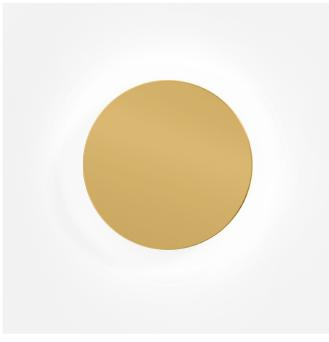
Disc shaped wall surface luminaire made from aluminium; Gold wet painted; brushed; PCB 3-step binning; phase-cut dim; light colour 3000 K; binning initial MacAdam  $\leq$  3 SDCM; CRI  $\geq$  90; 220 - 240 V; degree of protection IP20; Class 2; light source replaceable by Wever & Ducré or by a professional with explicit authorization;
