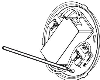
**3** Drill the marked holes with a diameter 6 mm.
