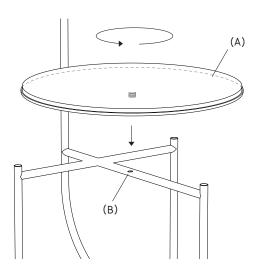
1. To assemble the Igram lamp-table screw the table top (A) onto the body (B).
