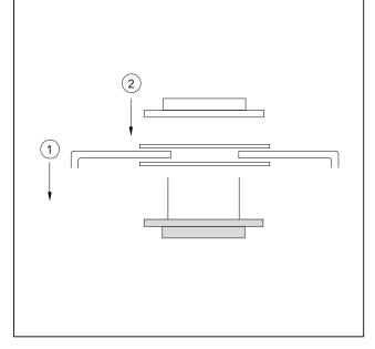
Place the lampshade on the frame (1) and fix with the second socketring on top. (2)
