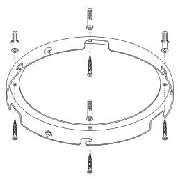
Drill four holes for the canopy bracket and one hole for each of the ceiling mounts.
