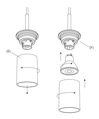
4. Unscrew the bulb socket housing (E) from the lamp body (F) and insert the light bulb into the bulb socket. Attach the housing back to the lamp body.
