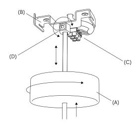
Connect the electrical cable with the terminal strip (C) then adjust the lamp height and tighten the cable (D). Attach the ceiling rose back to the ceiling mounting.
