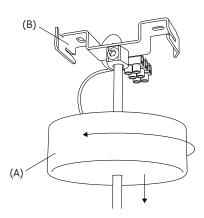
1. Remove the ceiling rose (A) from the ceiling mounting (B).
