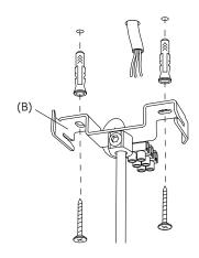
Mount the ceiling mounting to the ceiling with two appropriate screws and plugs. Always use correct screws and plugs for the mounting surface.
