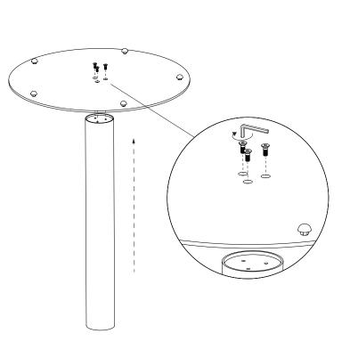
Mount the table base on the column with 3 (A) counter sunk screws.
