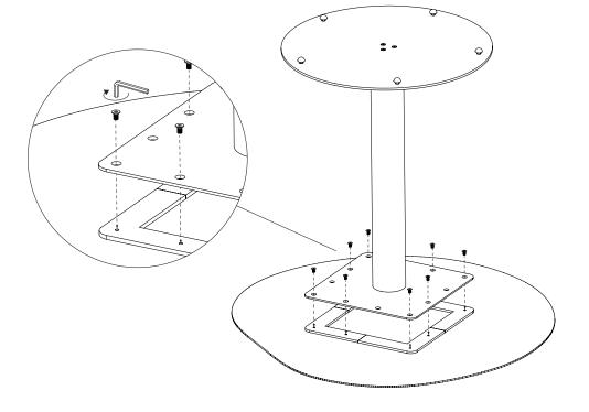
Mount the Connection plate on the column with 3 (A) counter sunk screws.
