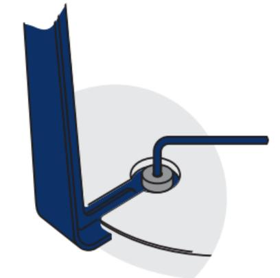
Tighten each screw with the provided Allen key.
