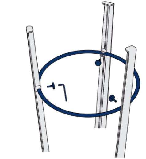
Put the ring on and tighten the 3 last screws with the Allen key.
