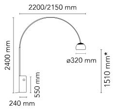
\*The diffuser can be adjusted to 1700 mm or 1850 mm.
